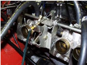
Revington TR have innovated and developed a new throttle improvement kit, which will fit all Triumph TR5 and 6 sports cars and Petrol Injected saloon models fitted with Lucas fuel injection.
