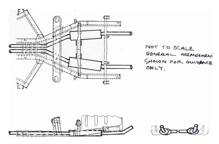
In many cases the ground clearance of this system is better than the standard TR5-6 system.
