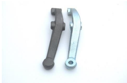
Figure 8: Raw forging with finished part
