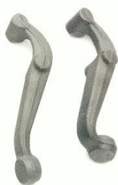
Figure 9: Raw forging with bent forging
