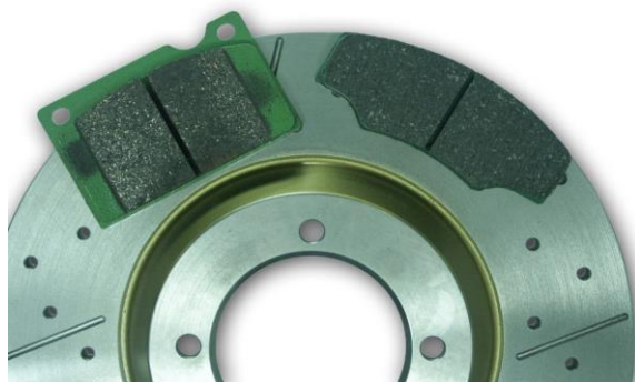
High performance peripheral pad to the right and with a conventional pad to the left
