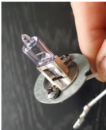
Figure 7: H3 bulb RTR8470 fitted to plate
