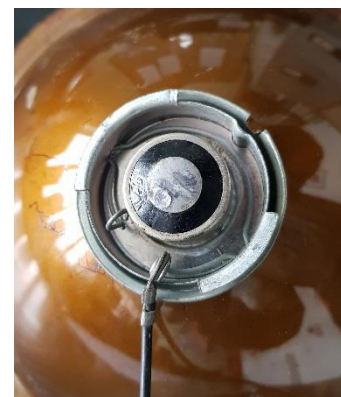
Figure 3: Standard or Halogen conversion bulb installed
