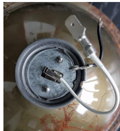
Figure 6: Assembly fitted into the holder retained by its clip
