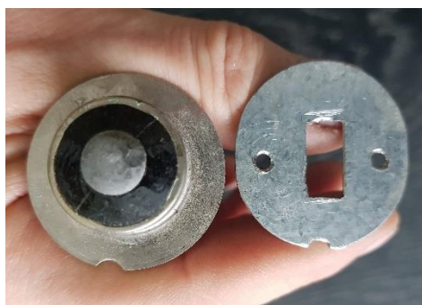
Figure 5: GLB323 on the left, Adaptor plate on the right
