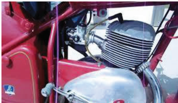
Peugeot 175 Bol d'Or, 2 Strokes with double exhaust
