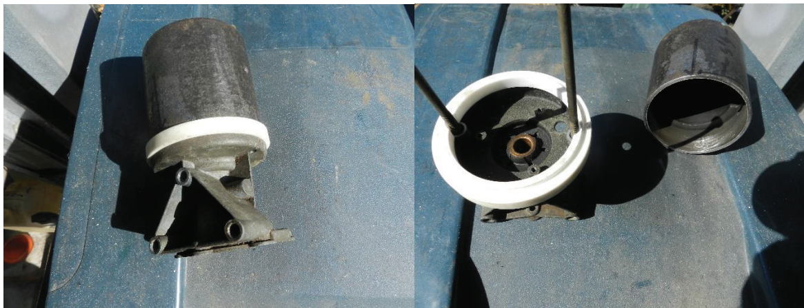
Shorten the motor on a lathe, an insulation block in methacrylate, and the heat is no longer transmitted. It's only common sense?
