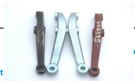
Figure 9: Raw forging with bent forging Figure 8: Raw forging with finished part Figure 7: Original parts with new parts
