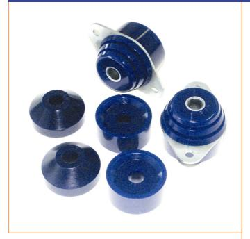
The differential mounting arrangement is a well-known weak point on the IRS TRs. The weaknesses inherent in the original chassis mountings are only compounded by the effects of tired rubber differential mounts – shock loads on acceleration, over-run and hard cornering do nothing to help matters.
