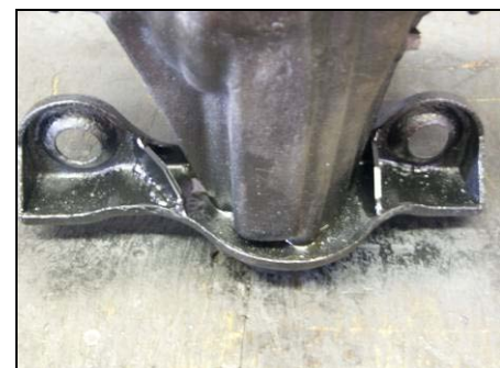
Figure 20: Item 1 Welded on the Front Mount
