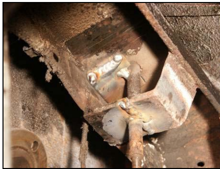
Figure 7: Half of Item 7 Welded in Place Under the Forward Bridge for Use with the Body Fitted
