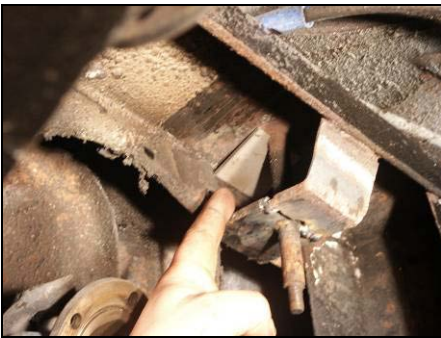
Figure 6: Half of Item 7 After Cutting Placed Under the Forward Bridge for Use with the Body Fitted
