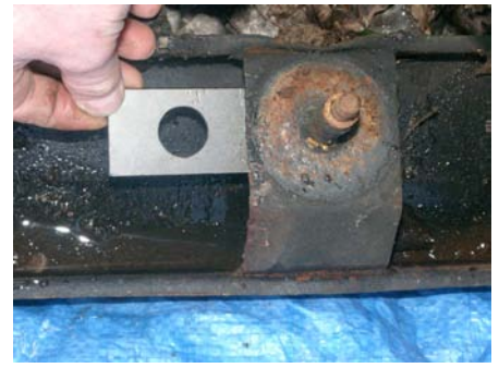
Figure 5: Item 7 Before Cutting in Half Placed Under the Forward Bridge for Use with the Body Fitted
