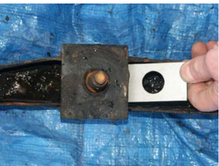
Figure 9: Item 7 Before Cutting in Half Placed Under the Rear Bridge for Use with the Body Fitted
