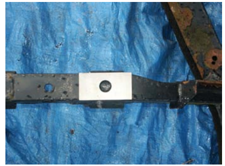
Figure 8: Item 6 Placed Above the Rear Bridge for Use with the Body Removed
